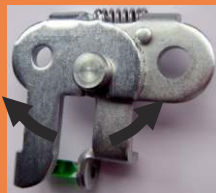
Separate the 2 parts and insert the glass phial
