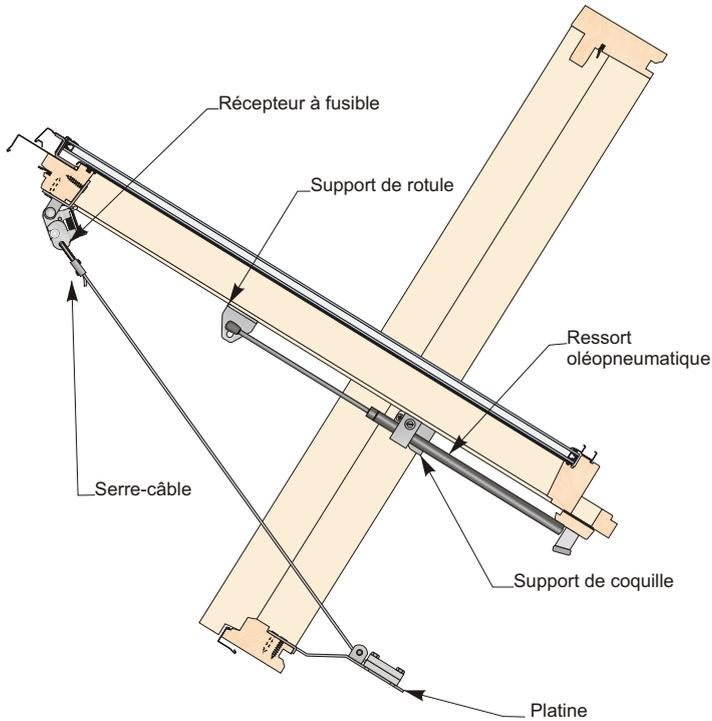
**MÉCANISME D'OUVERTURE MOV5000**
